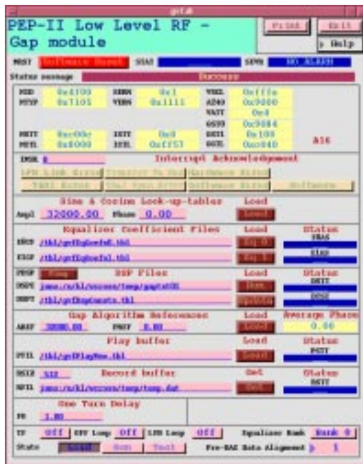
Figure 5: EPICS panel for Gap Voltage Feed-Forward Module control.
