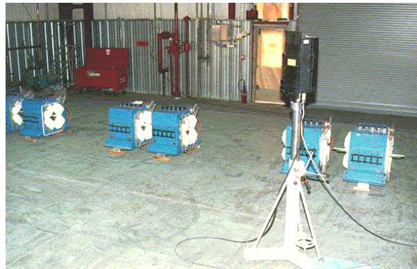
Figure 3 Six magnets ganged for fiducialization
