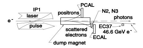
FIGURE 1: Schematic layout of the experiment.
