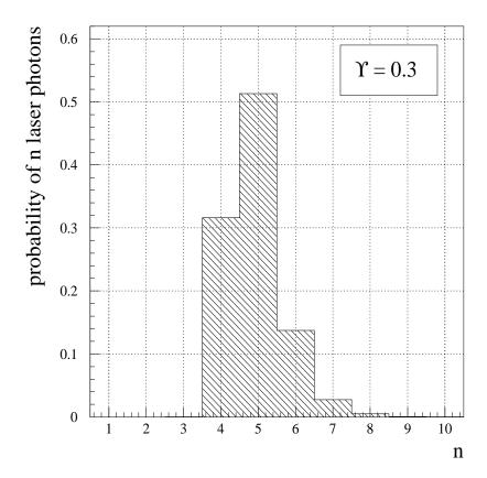
FIGURE 4: Calculated probability distribution of the number n of photons absorbed from the laser field in the second step of the two-step Breit-Wheeler pair creation process. A field intensity of  $\Upsilon=0.3$  at the laser focus was used for the simulation.
