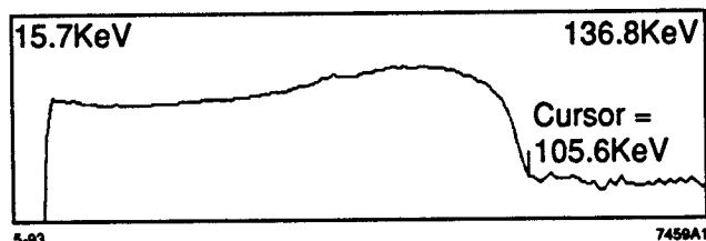
Figure 3. Energy distribution of emitted xrays for 110 kV.
