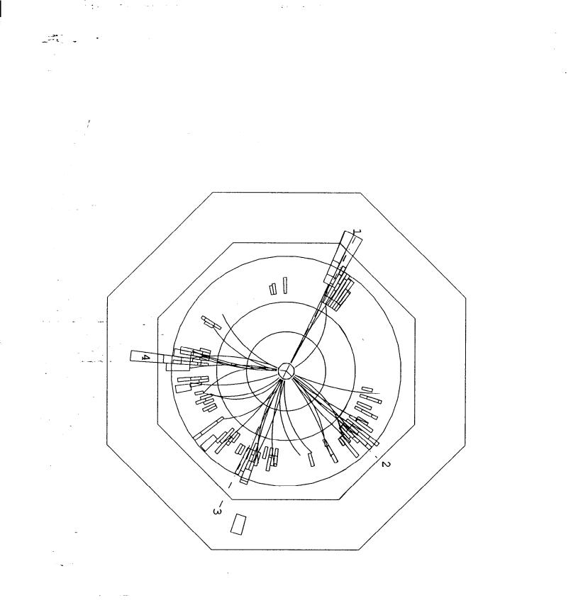
Figure 1. An event display, looking along the beam direction, of a neutral Z particle decaying into four "jets" of particles using the SLD detector at the Stanford Linear Collider. The curved lines are trajectories of charged particles reconstructed from the measurements in the inner cylindrical detectors, while the trapezoidally shaped boxes represent energy deposited in the outer detectors.
