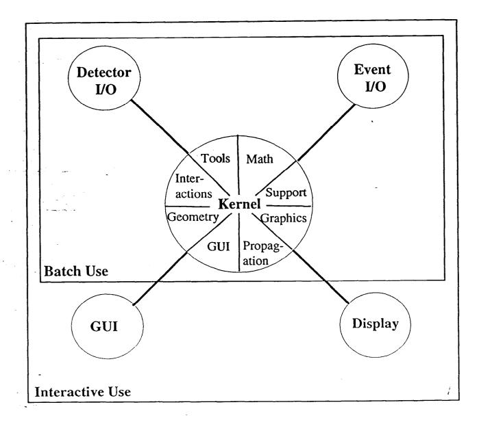
Figure 2. Illustration of the relationship of the Gismo kernel to detector and event I/O, the graphical display, and the graphical user interface.
