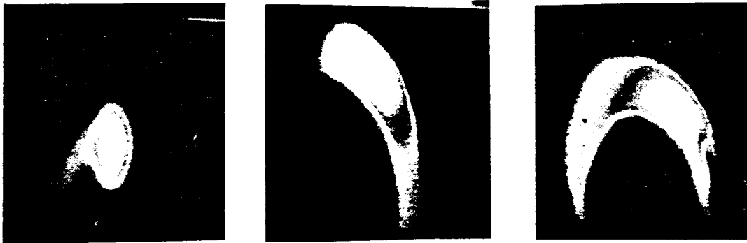
Fig. 9 Profiles (x-y) of a 2 \times 10^{10} e - bunch at 47 GeV with a 0.2 mm oscillation (left), with a 0.5 mm oscillation (center), and with a 1 mm oscillation (right) in both planes. The initial core sizes in both planes are about 120 \mu\text{m} .
