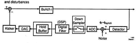
Fig. 1 Conceptual bunch-by-bunch, downsampled feedback system.
