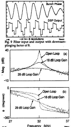
Frequency (kHz) 7285A1 Fig. 10 Magnitude (a) and Phase (b) response for a single bunch for open loop and closed loop gains of 18 and 28 dB.
