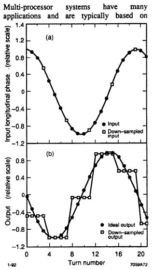
Fig. 4 Response of the downsampled filter with hold buffer. In (a), the squares are sampled values of the oscillation. (b) shows ideal and downsampled outputs to a kicker.
