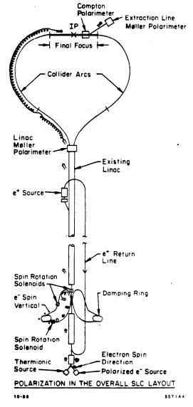
Fig. 1. Schematic of the SLC showing components of the polarized source, beam transport, and diagnostics. Spin orientation is indicated by the arrows.
