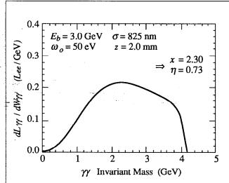
Figure 3. The two-photon luminosity distribution for a  $\sqrt{s} = 6$ , 8, and 10 GeV collider. In each case the laser wavelength has been chosen to tailor the photon spectrum to the 1.0-4.0 GeV mass region, and the beam spot size is assumed to come from relation (3). At the higher  $e^-$  beam energies the  $\eta$ parameter is smaller, resulting in larger luminosity at low invariant mass. Also note that at higher beam energies the required FEL photon frequency is reduced.
