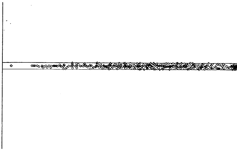
Fig. 21. Positron birthplaces in a wire target: 100 incident e^- , 793 accepted e^+ .
