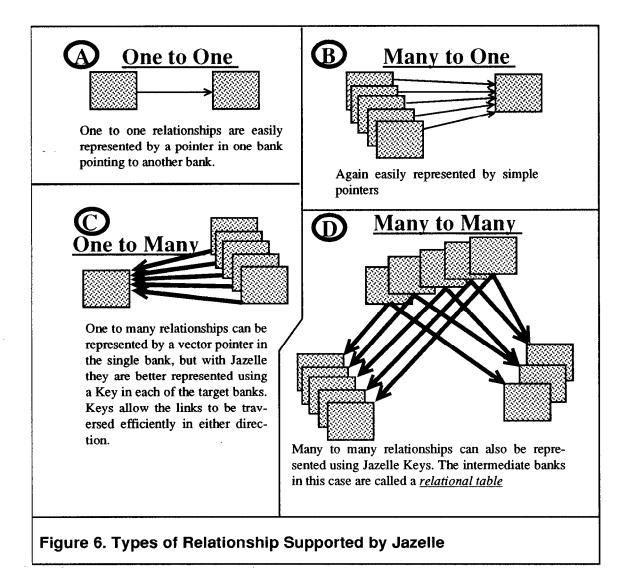
represent a completely arbitrary N by M relationship. The family of banks used to create the particle-vertex relational table is called PHPTVX, as is shown in Figure 7. Properties of the relationship, such as the distance of closest approach of the track to the vertex, are stored in the bank along with the keys which point to the track and vertex banks.
