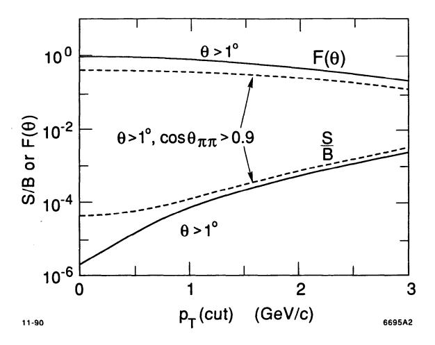
Fig. 3 - For the SSC collider the signal-to-background ratio (S/B) as a function of  $p_T(cut)$  for the  $B \to \pi^+\pi^-$  using also  $\theta$  and  $\theta_{\pi\pi}$  cuts (the two lower curves). Here  $\theta$  is the angle of the  $\pi^\pm$  with respect to the beam direction while  $\theta_{\pi\pi}$  is the opening angle between the two pions. The upper curves indicate the fraction of  $B \to \pi^+\pi^-$  (F( $\theta$ )) passing the various cuts.
