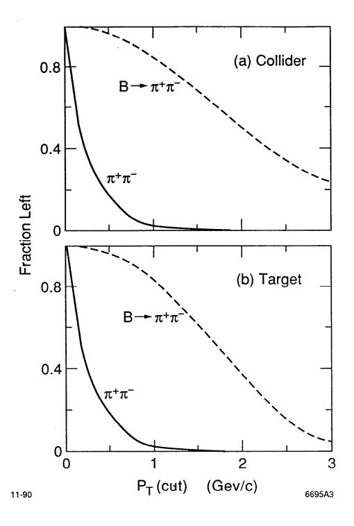
Fig. 2 - The fraction of  $B \to \pi^+\pi^-$  and  $\pi^+\pi^-$  background (see text) left after taking  $\pi^{\pm}$  having a momentum transfer greater than  $p_T(cut)$ . The SSC collider and target are represented by (a) and (b), respectively.
