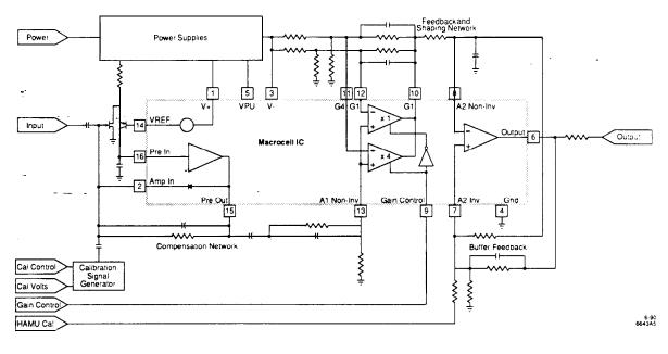
FIGURE 3. CRID preamplifier composed of macrocell amplifier and external JFET and surface mount components.
