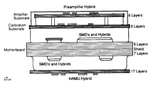
Cross section of a drift motherboard showing the main PC board with components and hybrids on both sides.
