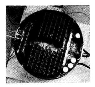
FIGURE 5 Photograph of a LAC "Top Hat" assembly. The cylindrical can is 13 cm high by 41 cm diameter.
