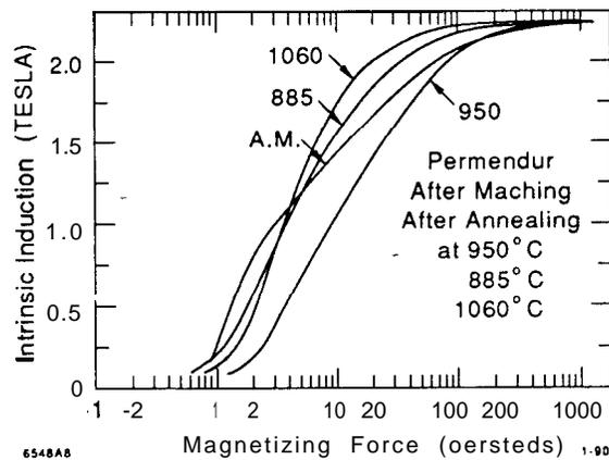
Fig. 8. Intrinsic Induction versus  $H$  for Permendur after machining and after annealing at three different temperatures.
