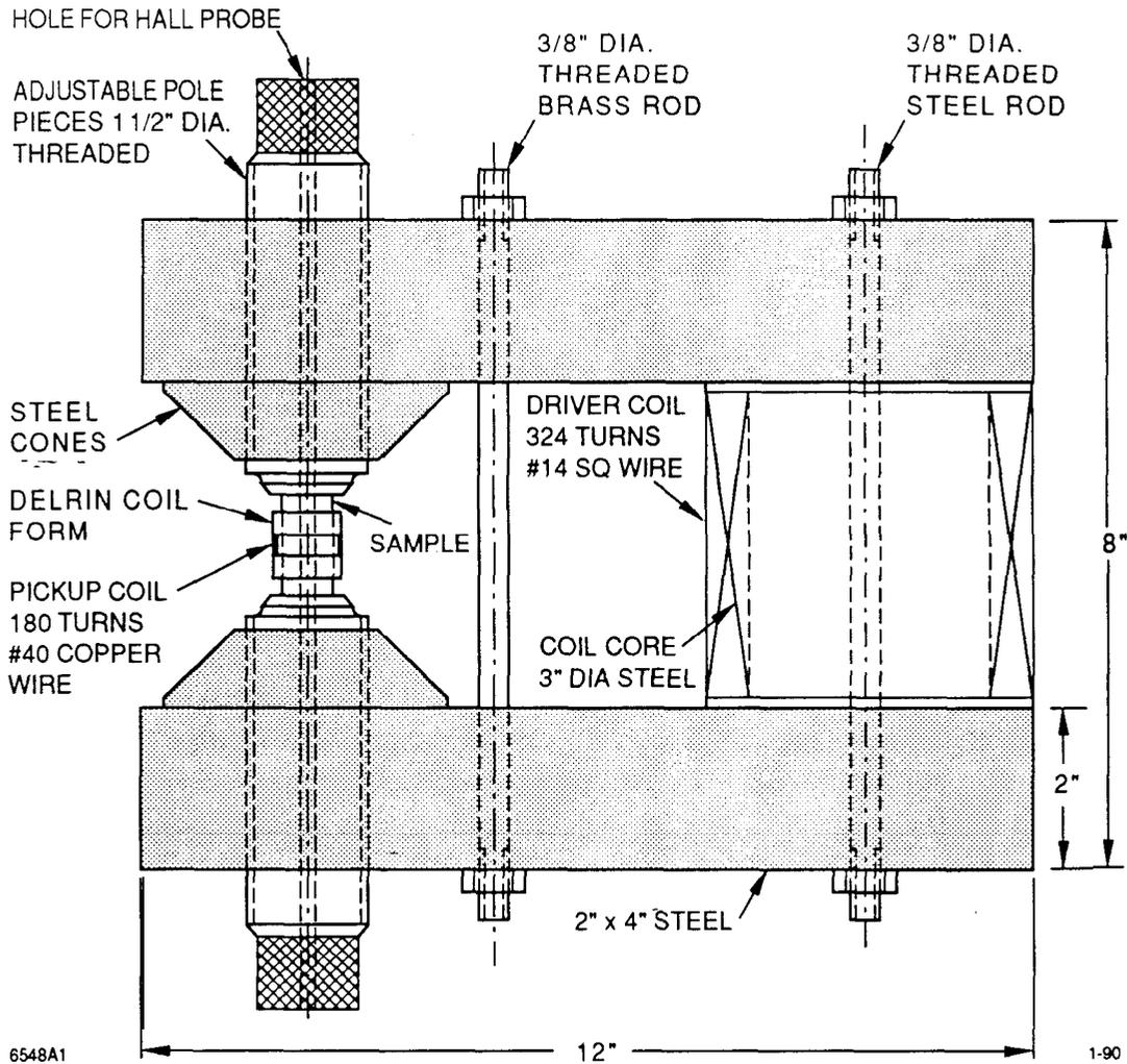
Fig. 1. Configuration of the SLAC Permeameter.
