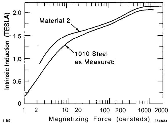
Fig. 4. Old POISSON table, and the new 1010 steel table.
