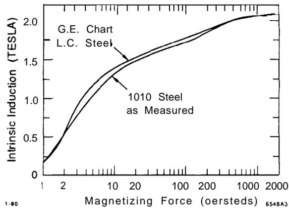
Fig. 3. Intrinsic induction ( $B-H$ ) versus magnetizing force  $H$  for annealed 1010 steel and low-carbon steel from the G.E. chart.
