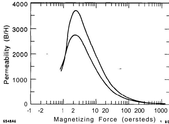
Fig. 6. Permeability versus magnetizing force  $H$  for annealed 1010 steel and Permendur.
