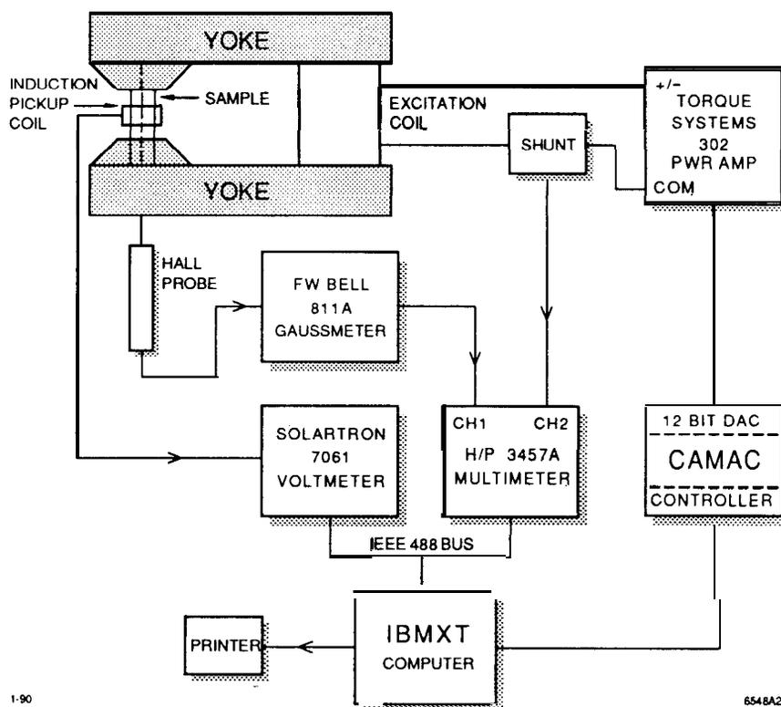
Fig. 2. The Permeameter measurement system.
