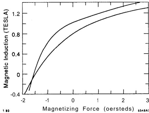
Fig. 7. Demagnetization curves for annealed 1010 steel and Permendur.
