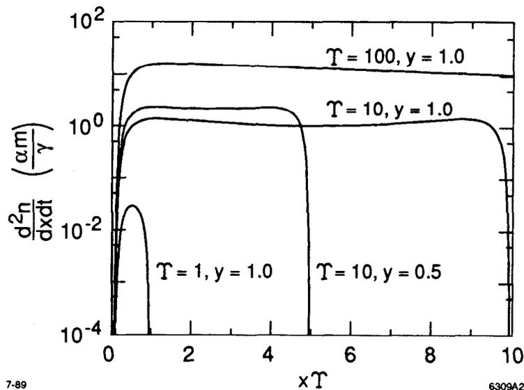
**FIGURE 2** Normalized spectrum for coherent pair creation, in units of  $\alpha m/\gamma$ , as a function of  $x\Upsilon$ . One sees that  $x_{min} \simeq 1/5\Upsilon$ .
