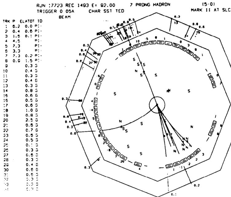
Fig. 14. Transverse view of the central drift chamber and octagonal liquid argon calorimeter for the first hadron observed by the MARK II at the SLC.
