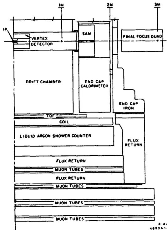
Fig. 9. Schematic representation of the MARK II.
