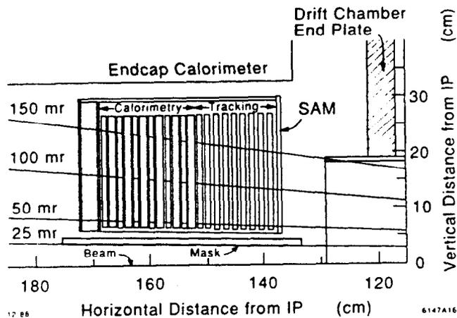
Fig. 10. Schematic drawing of a small angle monitor.
