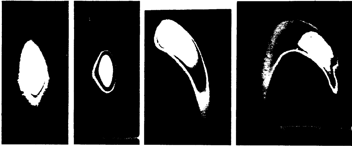
FIGURE 6 Images of an e^- beam on a profile monitor showing wakefield growth with increasing oscillation amplitude. The left image is for a well-steered beam and the right one for an oscillation amplitude of 1 mm. The beam intensity is 2 \times 10^{10} electrons. The core sizes \sigma_x and \sigma_y are about 120 \mu\text{m} .
