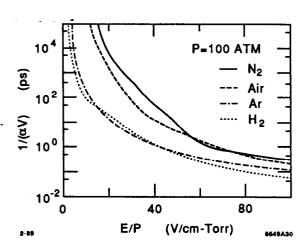
Figure 3:  $1/\alpha v$ , or time constant for avalanche growth, for different gases (Air, Nitrogen, Hydrogen, Argon), at a pressure of 100 Atm.
