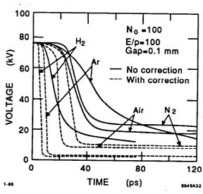
Figure 6: Effect of density correction on calculated waveforms.
