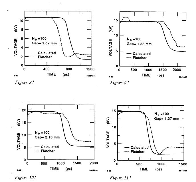
\* Figures 8-12: Comparison between calculated waveforms and Fletcher's oscillographic recordings. The dashed traces are obtained by digitizing the Physical Review figures enlarged ~ 10 times the original.
