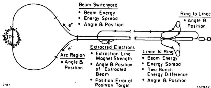
Fig. 1. Beam Stabilization loops in the SLC. The loops are clustered in a small number of regions along the accelerator and into the Arcs.
