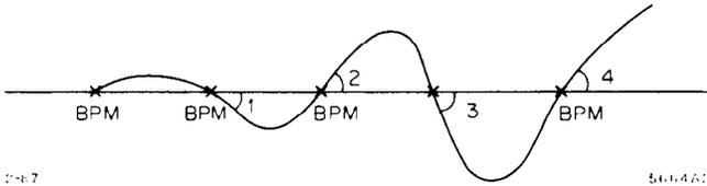
Fig. 2. Divergent orbit with increasing angle error if  $A > 1$ .
