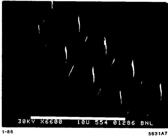
Fig. 6. Electron microscope photograph of our etched collonade structure for 10  $\mu\text{m}$  radiation.
