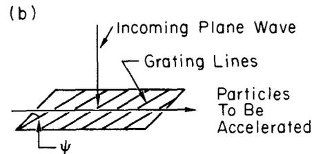
Fig. 1. Geometries of grating accelerators: a) as proposed by Takeda and Matsui; b) with skew grating to allow acceleration of relativistic particles; c) with skew initial wave as alternative to b).
