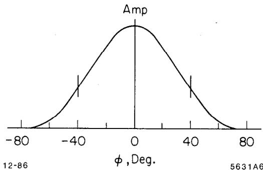
Fig. 7. Angular distribution of radiation to or from droplet structure.
