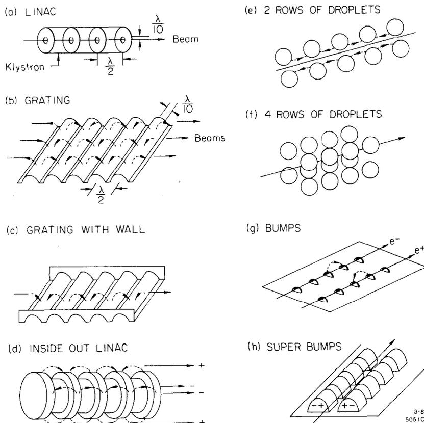
Fig. 4. New field accelerating structures.
