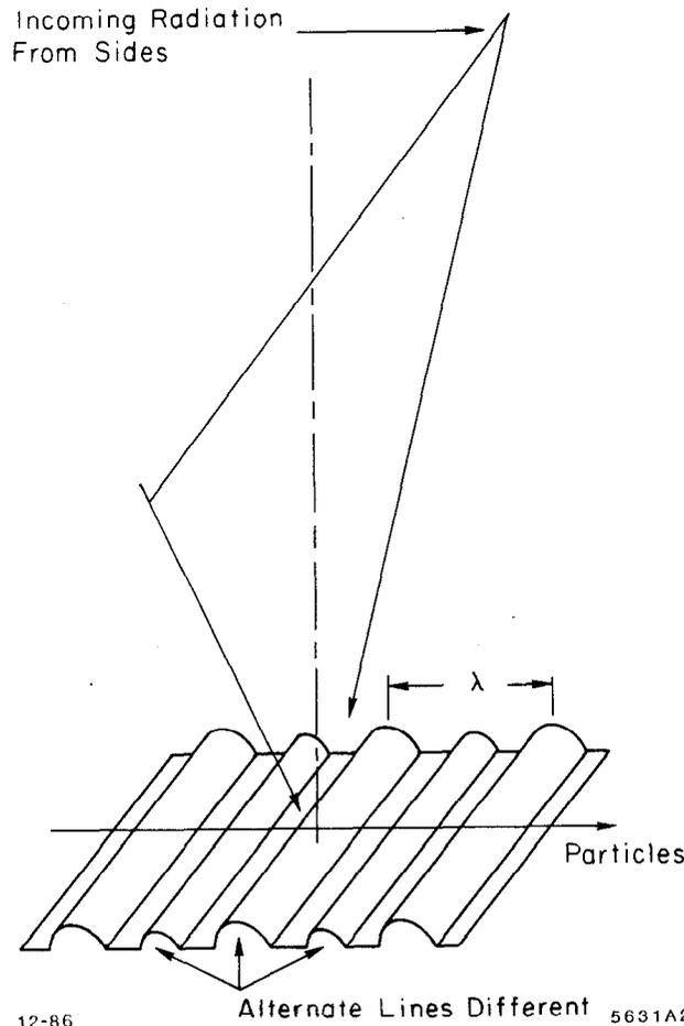
Fig. 2. Geometry of grating and incoming radiation showing perturbed grating lines to couple the radiation to the accelerating mode.
