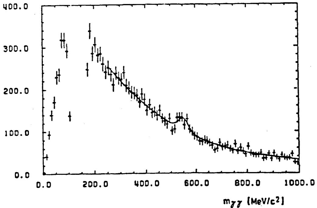
Fig. 12 The invariant  $\gamma\gamma$  mass spectrum. Pairs consistent with  $\pi^0$ s are subtracted.
