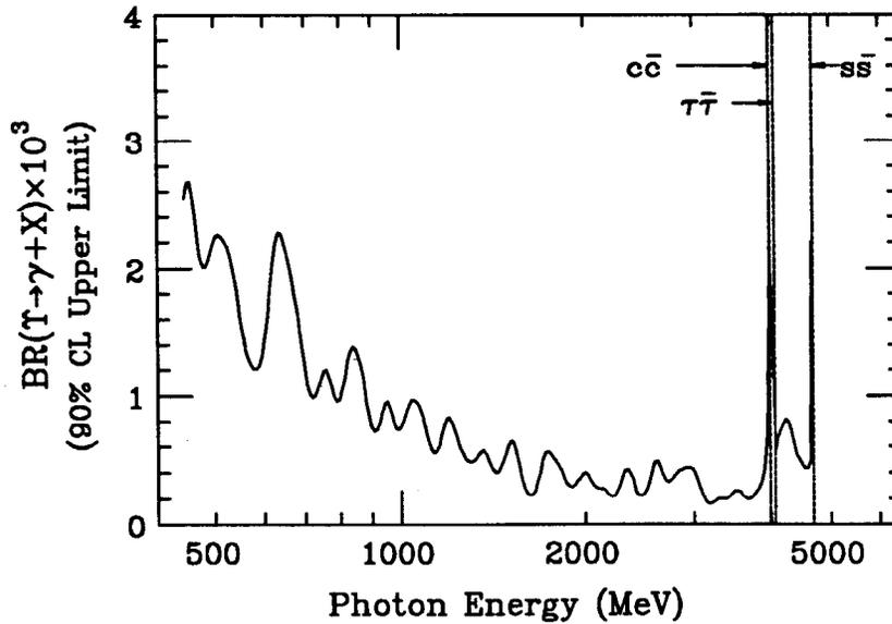
*Fig. 3* The 90% confidence level upper limit for the process  $\Upsilon(1S) \rightarrow \gamma X$  as a function of photon energy. The assumptions on the decay of  $X$  are found in the text. The vertical dashed lines show the kinematic thresholds for the relevant fermions.
