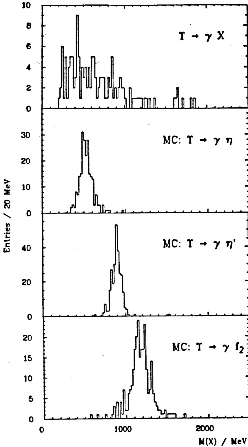
*Fig. 8* The top plot shows the observed invariant mass for the state  $X$  consistent with the process  $\Upsilon(1S) \rightarrow \gamma X$ . The other 3 plots indicate the mean and width expected for the corresponding decay mode calculated from Monte Carlo simulations.
