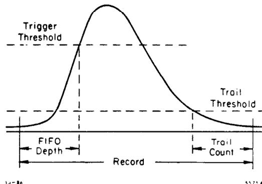
Fig. 2. WSM Compaction.
