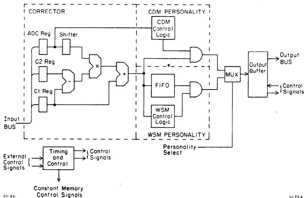
Fig. 1. Block DCU Block Diagram.
