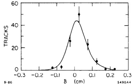
Figure 4. DELCO impact parameter distribution for electron tracks used to determine  $\tau_b$ . The points with error bars are the data. The smooth curve is a Monte Carlo calculation based on the measured value of  $\tau_b$  and the resolution used in the maximum likelihood fit.
