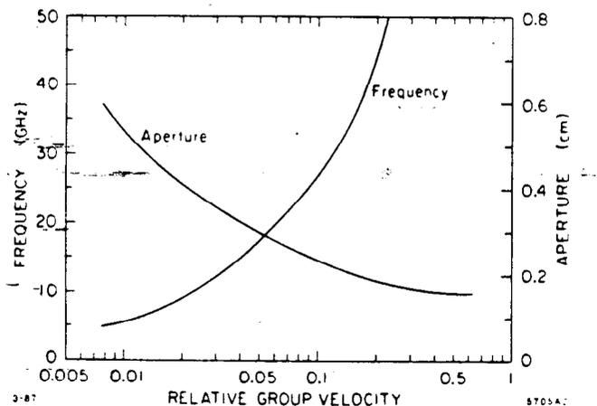
Fig. 3. Frequency and aperture with  $\tau = 0.61$ ,  $L = 1$  m versus relative group velocity.
