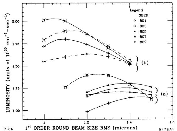
Fig. 4. Luminosity versus first order beam size: (a) for a momentum spread of  $\delta = 5 \times 10^{-3}$ ; and (b) for a momentum spread of  $\delta = 2 \times 10^{-3}$ .
