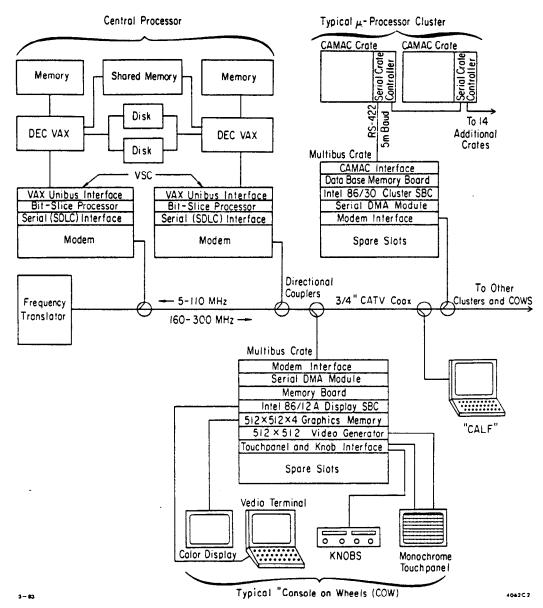
Fig. 4. The SLC computer control system.
