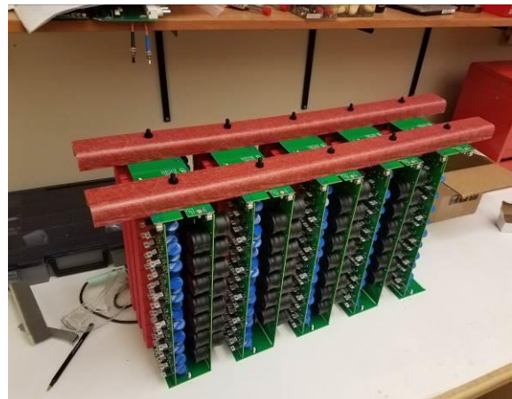
Fig. 1. Photograph of an inverse Marx topology energy recovery modulator for the CPI VKS-8262S. The Marx has 5 stages and will be connected to a 4-stage depressed collector.
