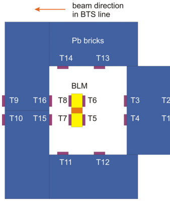
Figure 1: Plan view of TLD placement on the BLM and Pb shield.
