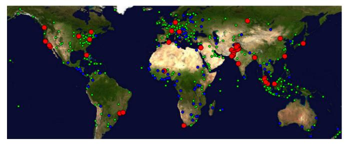
Fig. 1. Locations of PingER MAs and remote sites as of June 2015. Red sites are MAs, blue sites are beacons that are monitored by most MAs, and green sites are remote sites that are monitored by one or more MAs.
