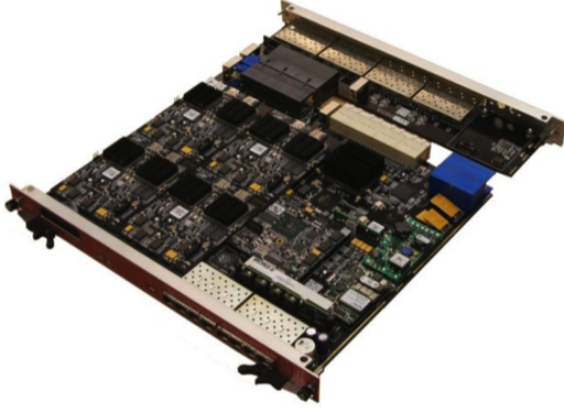
Fig. 12. One COB ATCA blade used in the RCE platform.
