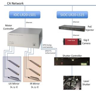
Figure 2: Hardware architecture for installation.
