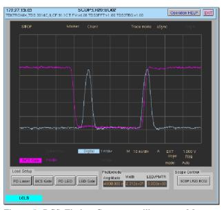
Figure 5: BCS Timing Gate on oscilloscope. Magenta trace shows the toroid timing gate and the blue trace shows the two laser pulses.
