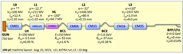
Figure 1: LCLS II Beamline Diagram
