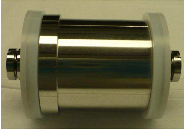
FIG. 2. Top: Photograph of the assembled xenon pump. Bottom: Photograph of the piston removed from the pump.
