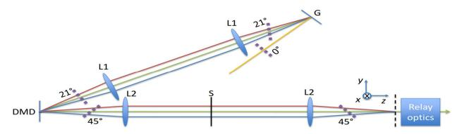
Figure 1: Schematic layout of optic design for the proposal of SLAC Compton scattering FEL. Where G means grating, L1, L2: lenses, DMD: digital micromirror device, S: slit. The yellow line represents an input fs pulse, red line chief ray of the longest wavelength  $\lambda_l$ , green line chief ray of the central wavelength  $\lambda_c$ , blue line chief ray of the shortest wavelength  $\lambda_s$ . The black dash line represents the image plane and the purple dash line the pulse front.
