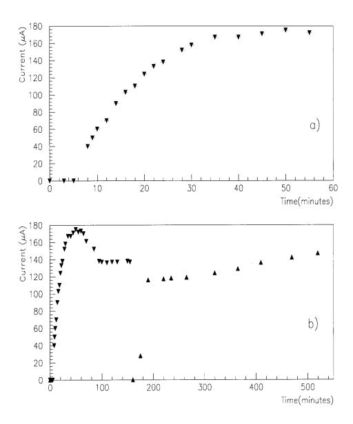
Figure 1: a) Short-term time dependence of current in straw #2 at 2.30 KV in pure  $CF_4$  gas; b) Long-term time dependence; the copper began to thin visibly from the tube wall somewhere between 410-470 minutes on this plot. These data were taken over two days and the second set begins at t=160 minutes.
