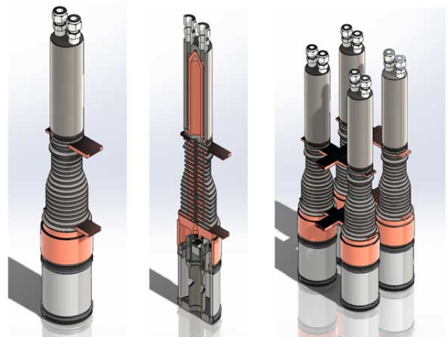
Figure 2. Mechanical Model of an Individual Klystron and Four Klystron MBK.
