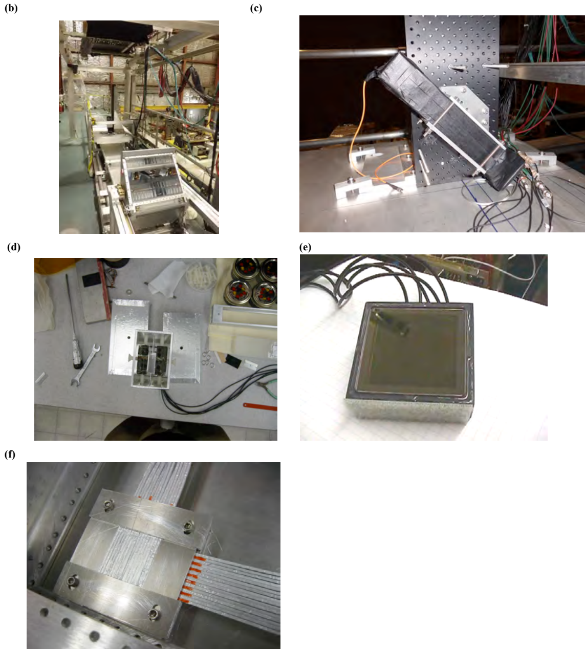
Fig. 5 Cosmic ray telescope (CRT) [11]: (a) Overall view of stack of iron and lead, interleaved with large scintillator paddles, tracking hodoscopes, start counter and FDIRC prototype. (b) FDIRC prototype in CRT, without electronics at this stage. (c) Start counter consisting of two fused silica bars and MCP-PMT detector. (d) The two start counter fused silica bars viewed from the end. (e) Burle 4-pixel MCP-PMT is an early R&D version, not produced any more. (f) 16x16 fiber hodoscope with 2 \times 2 \text{ mm}^2 scintillating fibers.
