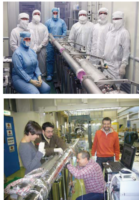
Figure 1: String assembly of four TESLA-type cavities by DESY/FNAL/KEK team (top), and tuner assembly by INFN/FNAL team (bottom).
