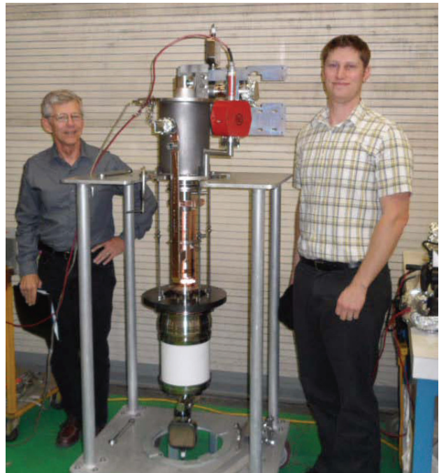
Figure 4: The LLNL XL4 klystron awaiting final testing at SLAC.
