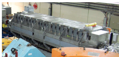
Figure 1: PS main magnet with a LHC-type BLM (yellow cylinder on top of the magnet) and an ACEM (orange cylinder in front of the magnet).
