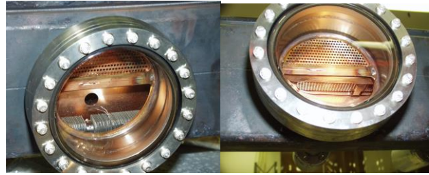
Figure 43: (left). Test module for the NEG pump. The wires leading from the pump material are a thermocouple. Figure 44: (right). The same chamber showing two different screen designs. The more difficult screen to see is a square hole design that proved to be more susceptible to letting HOM power into the pumping chamber.
