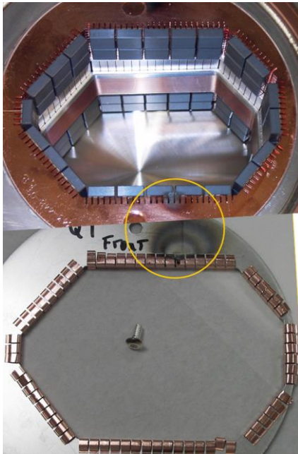
Figure 36: Q2-bellows and \Omega -seal with traces of sparking.
