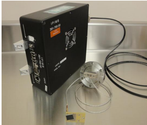
Figure 3. Photograph of the prototype Intensity Monitor with PGP (IMP) to readout photodiodes (left). The photograph on the right side show the commercial x-ray photodiode used for the measurements. A sheet of 30 \mu\text{m} Kapton is glued in front of the diode to block optical light.
