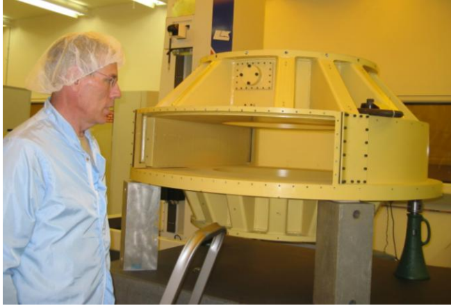
Figure 7 Left the body of the corrector which houses lenses C4-C2, the filter changer and the shutter. Right: the conical piece of the corrector which attaches to the body and supports C1. Inspection of the delivered parts is currently in progress at Fermilab.
