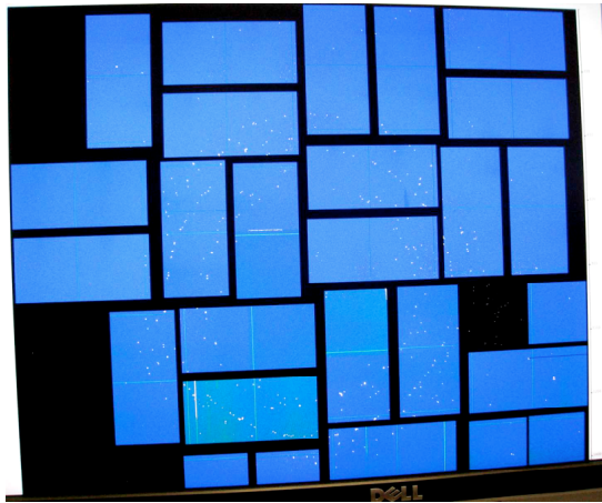
Fig.2: Screen shot of the LCLS-CXI camera showing unresponsive ASIC (black square on the lower right) and white spots in a circular pattern so-called water rings.
