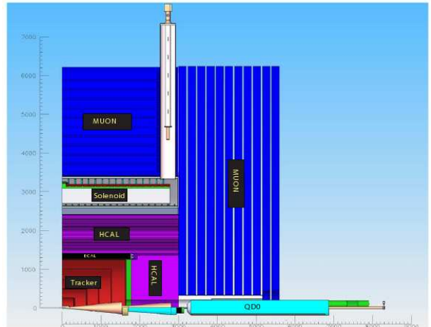
FIG. 1: Disposition of subdetectors in SiD quadrant. All dimensions are in mm.
