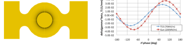
Figure 2. Quadrupole fields in the dual-feed input coupler with a cylindrical cell profile.
