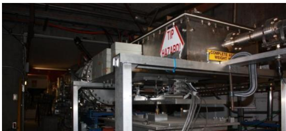
Figure 7: Collimator wakefield chamber test allows an exchange of collimators and adjustment of jaw aperture [8,9].
