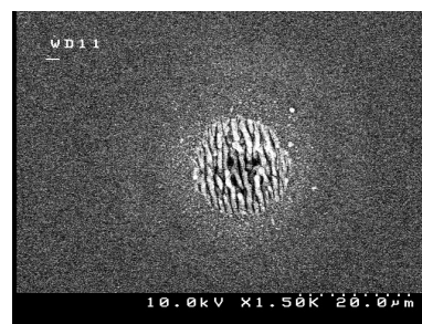
Figure 2: An SEM image of a typical test site after laser-induced damage. The fringe pattern is characteristic of multi-shot laser damage.
