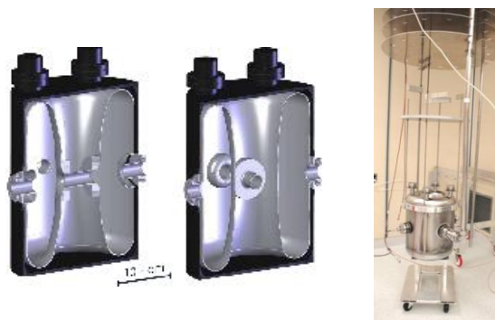
Figure 1 Beta 0.53 superconducting half-wave resonator cavity for the FRIB. Left: schematics of the HWR cavity; Right: Niobium prototype of the HWR cavity.
